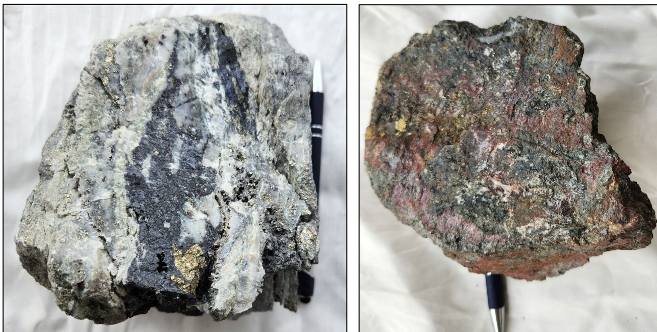
Photos 5 & 6. Float sample of a 10cm chalcedonic, banded quartz vein with sphalerite, arsenopyrite and pyrite that returned assays of 33.3g/t gold, 37.4g/t silver & 5.6% zinc ( LHS ) & a float sample of diorite with chalcedonic quartz veins and quartz vein breccia with disseminated chalcopryite and possibly cuprite that returned assays of 44g/t gold, 119g/t silver & 1.1% copper ( RHS ).
