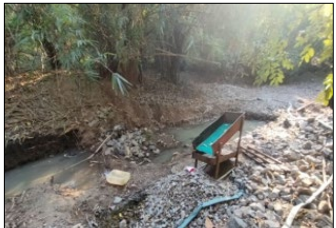
Photos 3 & 4. Recent alluvial artisanal gold workings at Ngot. Gold mineralised quartz vein gravels are located in a 50cm wide band approximately 1m below surface.
