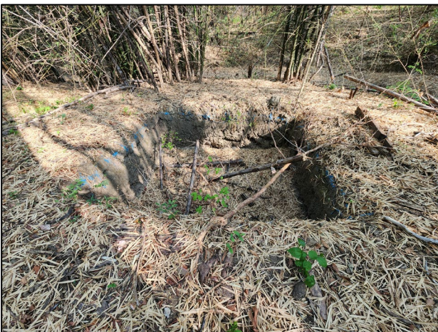
Photos 3 & 4. Recent alluvial artisanal gold workings at Ngot. Gold mineralised quartz vein gravels are located in a 50cm wide band approximately 1m below surface.
