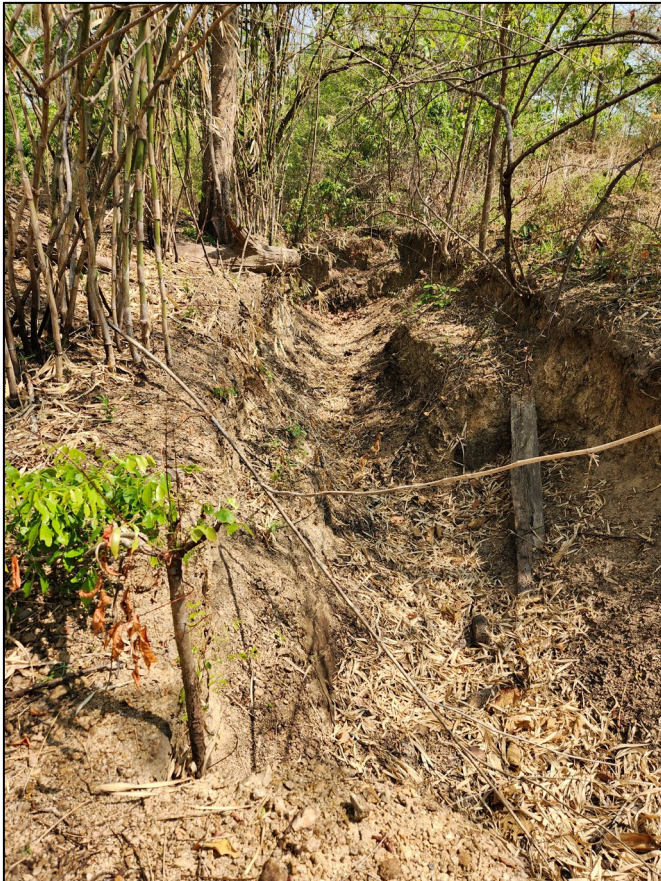
Photos 1 & 2. Historical artisanal gold workings (+5 years old) on primary mineralisation hosted in diorite (LHS) & a historical artisanal mining cyanide leach pad (RHS).
