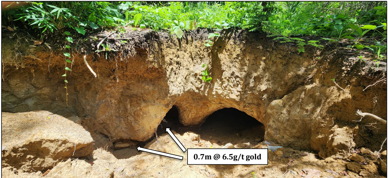
Photograph 1. Ngot Central Prospect – new artisanal workings on shallow-dipping, stacked high-grade gold veins hosted in weathered diorite (5m below surface).
