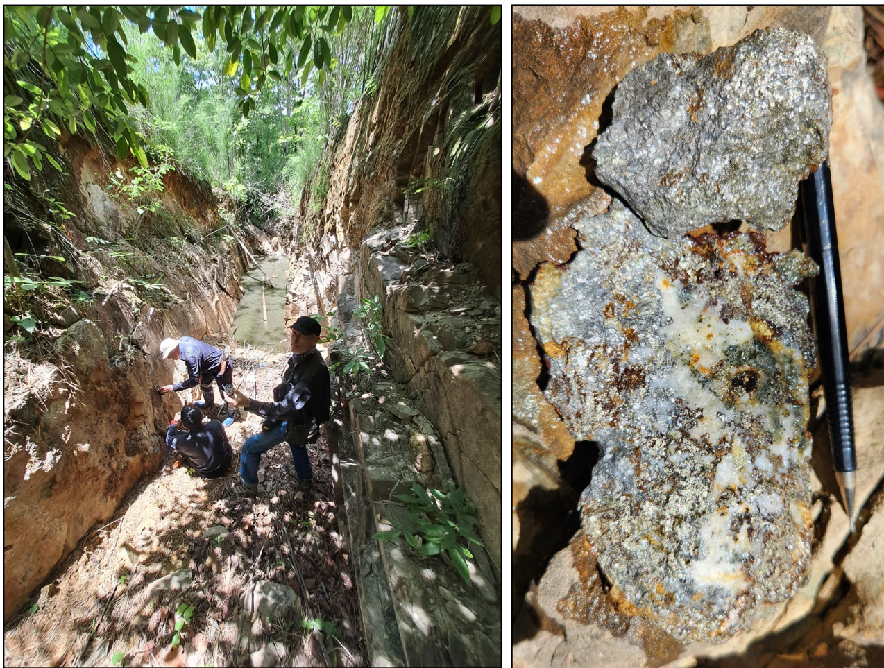
Photographs 4 & 5. Srolao Prospect – 40m long x 2m wide x 3-7m deep slot that trends east-west ( Left ) & remnant quartz-arsenopyrite-pyrite-hematite vein mineralisation from the footwall of the workings. The mineralisation strikes 080^{\circ} and dips 76^{\circ} S and assayed 27.4g/t gold, 5.1g/t silver & 30.1% arsenic ( Right ).
